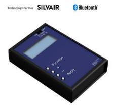
Operationally, each MESH-SCHD can be provisioned to the same network as the MESH-CTRL products and be used to control a group of MESH-CTRL lighting controllers. Each controller in the group is dimmed to, and maintained at, the desired % intensity from a Bluetooth® mesh command from the MESH-SCHD. For 0-10V drivers with dim-to-off capability, an intensity level of 0% turns the fixture off.
